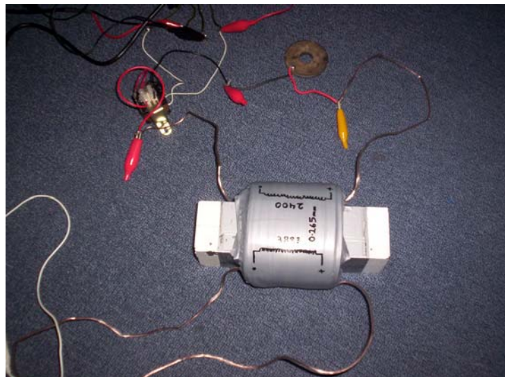
New MRA winding for higher power
