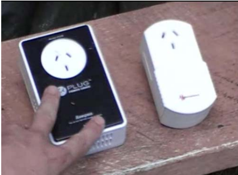
A power saver (left) and a dirty electricity filter (right)
